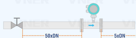
HALF OPENING VALVE OF REGULATING VALVE
